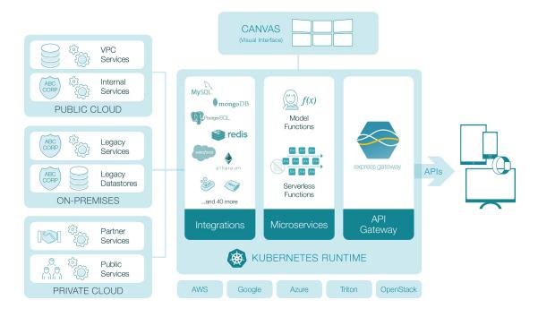
Express Serverless Platform can be installed on bare metal, VMs, or any managed Kubernetes offering with all the necessary infrastructure components included: an API Gateway, Kubernetes Based Runtime, Serverless Engine and visual Canvas that serves as a "single pane of glass" to visualize your microservices and API development.
